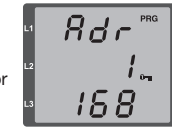
Fig. TCP/IP address, Byte 1, value 168. A TCP/IP address consists of 4 bytes with the following structure (example):
