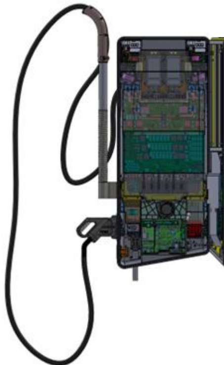
Figure 1: HYC_50 with open front door (Example with one DC charging cables)
