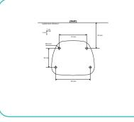
Use included template (or print out from downloaded manual) to drill 4 hole for the wall
