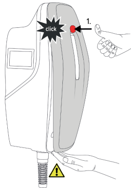
Fig. 18: Attach front cover (example) - 1
